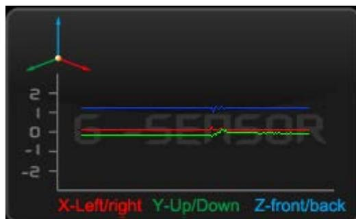
**G-SENSOR** : Gravity Sensing Analysis, When Triggering G-Sensor Forced Video Recording, Data of X, Y, and Z Axis Changes of the Vehicle will display.
