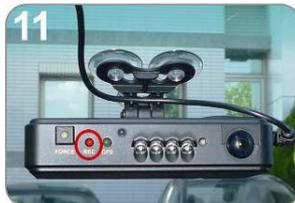
11 Red: flashing during recoding, Fast flashing in emergency mode.
