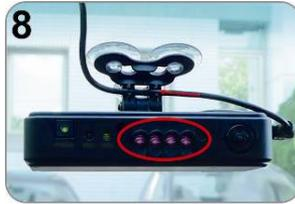
8 When the power is successfully connected, the IR LED will light on for 10 sec.
