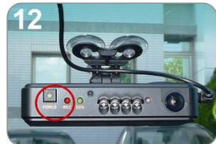
12 Force Record Button: When press down, the red light will flashing rapidly. In the night its LED will light on as indicator.
