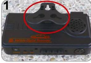
1 Make the bracket facing upward.
