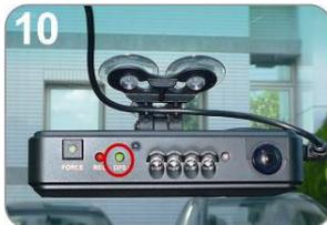
10 Green: flashing while GPS is positioning, Light on when GPS is ready.
