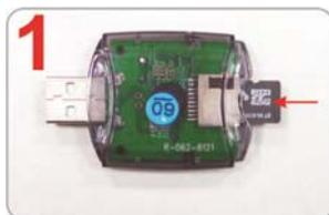
Insert the Micro SD card into the card reader (Please make sure the direction is correct)
