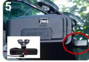
5 Plug the power cable to socket on photo No. 5 or No. 6, please do not plug in both sockets at the same time)
