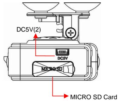
※ Please do not plug the power in both micro-USB terminals. The machine might be damaged.
