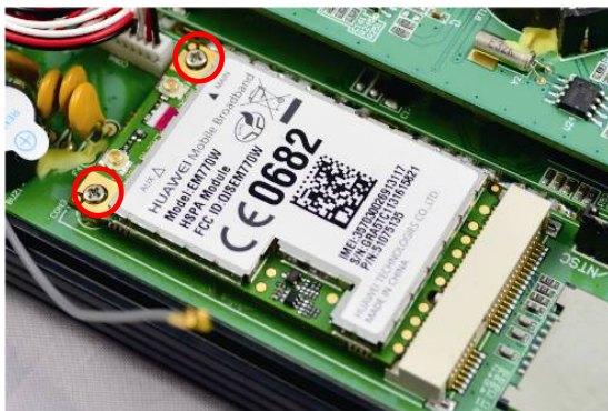
3. Two pieces of M2 screws Locked on the 3G module.
