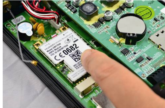
2. Flat press the 3G module on the mother board.
