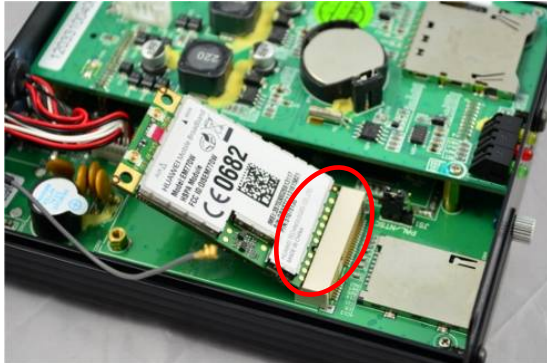
1. The 3G module is sloped to plug into slot of PCI-E
