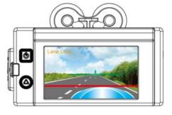
4. Use the keys of remote controller to adjust horizontal line above engine cover. When the line can be recognized by VVR, "Lane Lock" will appear.
