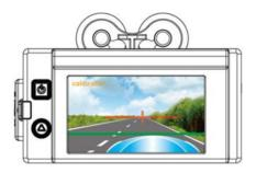
3. Use the keys of or remote controller to adjust the "CROSS" in the exact middle of the road. If setting fails, "Can't get Lane" will be appeared. Use to change horizontal line.
