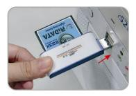
2. Insert the reader into the USB Port on PC.
