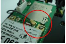
4. Complete installation of antenna and module
