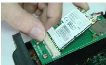
1. Slanting insert the 3G module into PCI-E slot.
