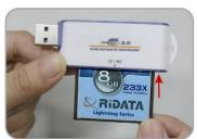
1. Put CF card into the reader slot and make sure the direction is correct.
