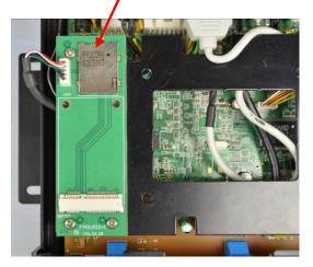
Installation interface for SIM card and 3G module.
