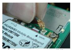
3. Connect antenna to "M" Position of the module
