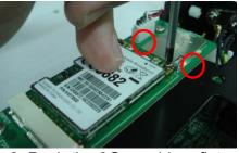
2. Push the 3G mould on flat status and lock two pieces of M2 screws.
