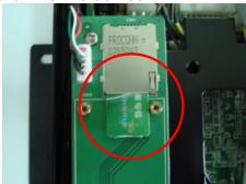
1. Insert SIM card into the slot
