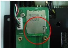
2. Flat the SIM card and push into the buttom then locked
