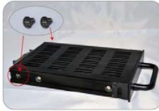
1. Remove the side screws of HDD tray.
