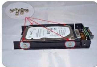
4. Fasten 4 screws to lock HDD in place.
