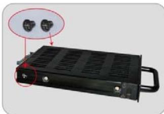
6. Fasten the side screws to complete HDD installation.
