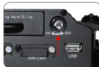
7. Slide the HDD tray back on DVR and lock the HDD in place (turn to ON).
