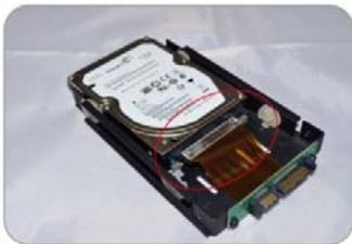
3. Connect HDD to SATA flat cable, align HDD with silicon buckle and slide in.
