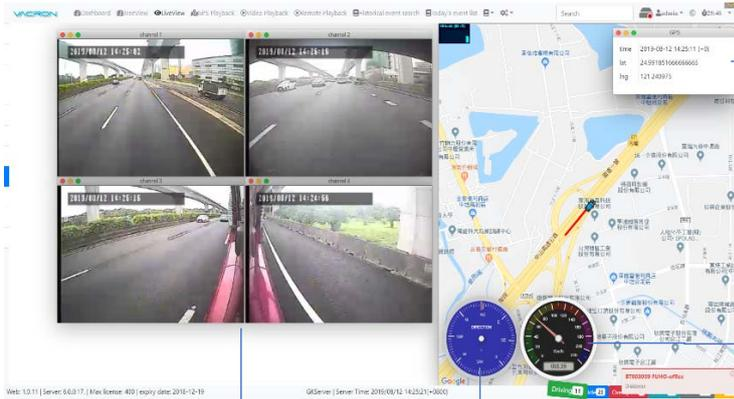
The screenshot shows a dashboard with four live video feeds of a road from different camera angles. To the right is a map showing the vehicle's location. Below the map are speedometer and direction indicators. A data popup is visible over the map.
