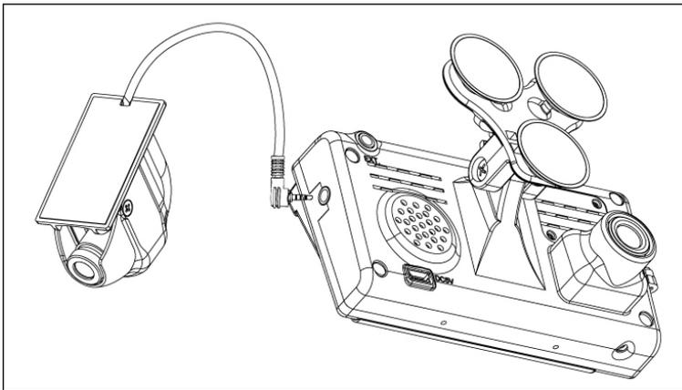
**Note: To avoid camera damage, please power off the vehicle video recorder before plug the camera in.**
