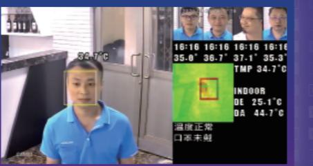
**Temperature measurement of thermal camera.**
