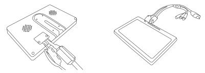
To avoid electromagnetic interference, please apply a powdered iron core about 3 cm close to the product end of the VGA wire, and round the composite video connector wire at the powdered iron core.
