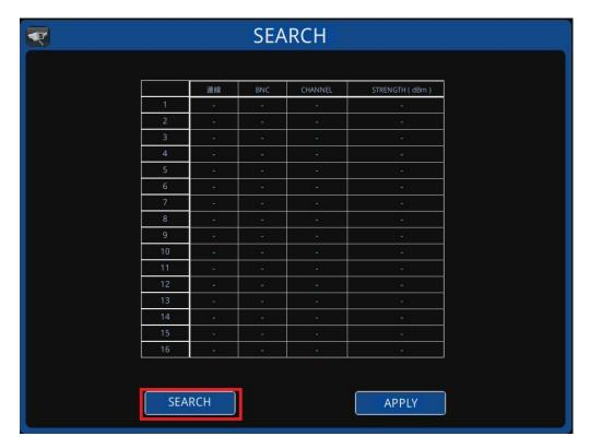
2) Owing to the RF interference of ccHDtv cameras, more cameras may be found than the connected ones. Then you can use 【AUTO SELECT】 to judge the usable cameras.
