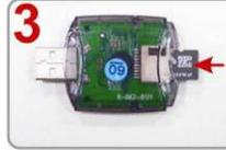
3 Insert the Micro SD card into the card reader (please make sure the direction is correct).
