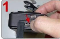
1 Turn the rubber cover left and press the Micro SD card with your finger to pop up.
