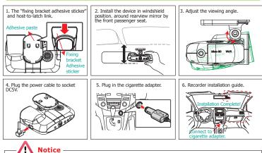
(1)Make sure that the front install your windshield is clean and dry. And install on a flat glass,
