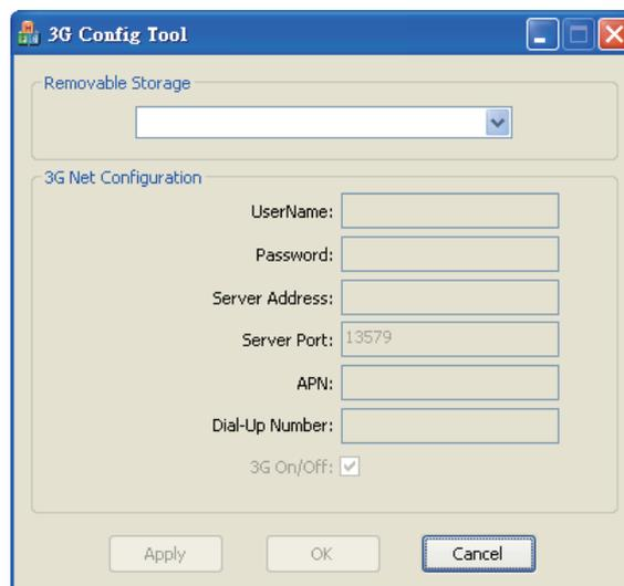
**Step 2. Then insert the SD card into the computer, select the SD card disk, and enter the relevant parameter settings.**
