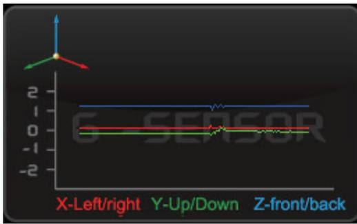
G-SENSOR : Gravity Sensing Analysis, When Triggering G-Sensor Forced Video Recording, Data of X, Y, and Z Axis Changes of the Vehicle will display.
